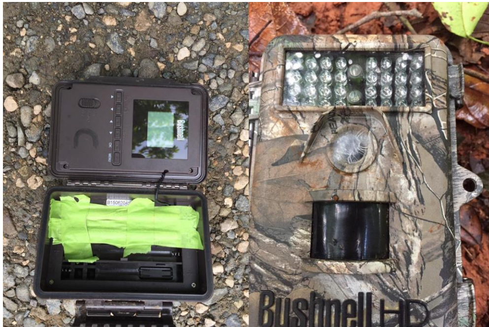
On the left Bushnell Model 2016 under “treatment” to keep batteries in place and spider web in lens on the right
