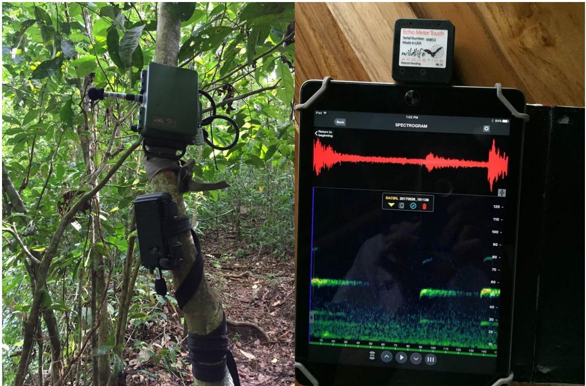
Some of the recording equipment: left SM4 bat and ARBIMON recorders, Bat Echo Meter on the right
